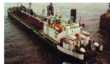
Ship name: "Thames" Owner: Prins van Vijnngaarden Type: Split barge/suction dredger Units: Ulstein Aquamaster ALT 400 azimuth thrusters Yard: IHC Holland, Holland
