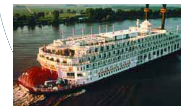
Ship name: "American Queen" Owner: Delta Queen Steamboat Type: River Cruise vessel Units: Ulstein Aquamaster US 901 CRP azimuth thrusters Yard: McDermott, USA
