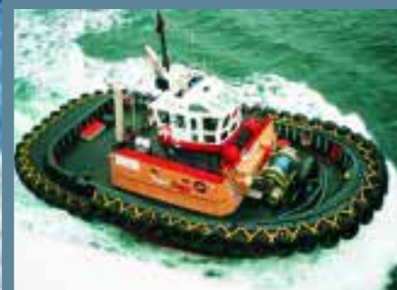
Ship name: "Tiger Sun" Owner: Tiger Tugs Rivtow Marine Ltd. Type: Harbour tug Units: Ulstein 1350H azimuth thrusters 2 x 1650H azimuth thrusters Yard: Sylte Shipyard Ltd.
