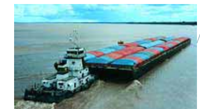
Ship name: "Sapezal" Owner: Hermasa Navegacao da Amazonia Type: River pusher Units: Ulstein Aquamaster US 1401 azimuth thrusters Yard: Erin Shipyard, Brazil
