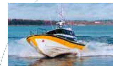
Ship name: "Victoria" Owner: Svenska Sjöräddningssällskapet Type: Fast rescue vessel Units: Kamewa FF375 water jets Yard: Malö Yachts, Sweden
