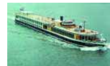
Ship name: "River Queen" Owner: Kamphuisen Type: River Cruise vessel Units: Ulstein Aquamaster US CRP 901 azimuth thrusters Yard: De Hoop Lopith, Holland
