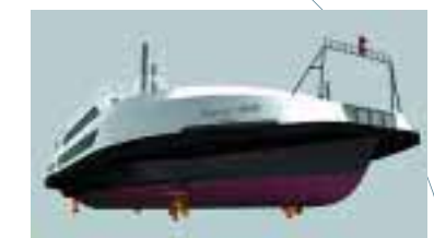
Ship name: "Osprey 2000" Owner: Kootenay ferry Type: Double-ended ferry Units: Ulstein Aquamaster 1350 H azimuth thrusters Yard: Kootenay Lake Ferry Builders Ltd. (Vancouver Shipyard Ltd.)
