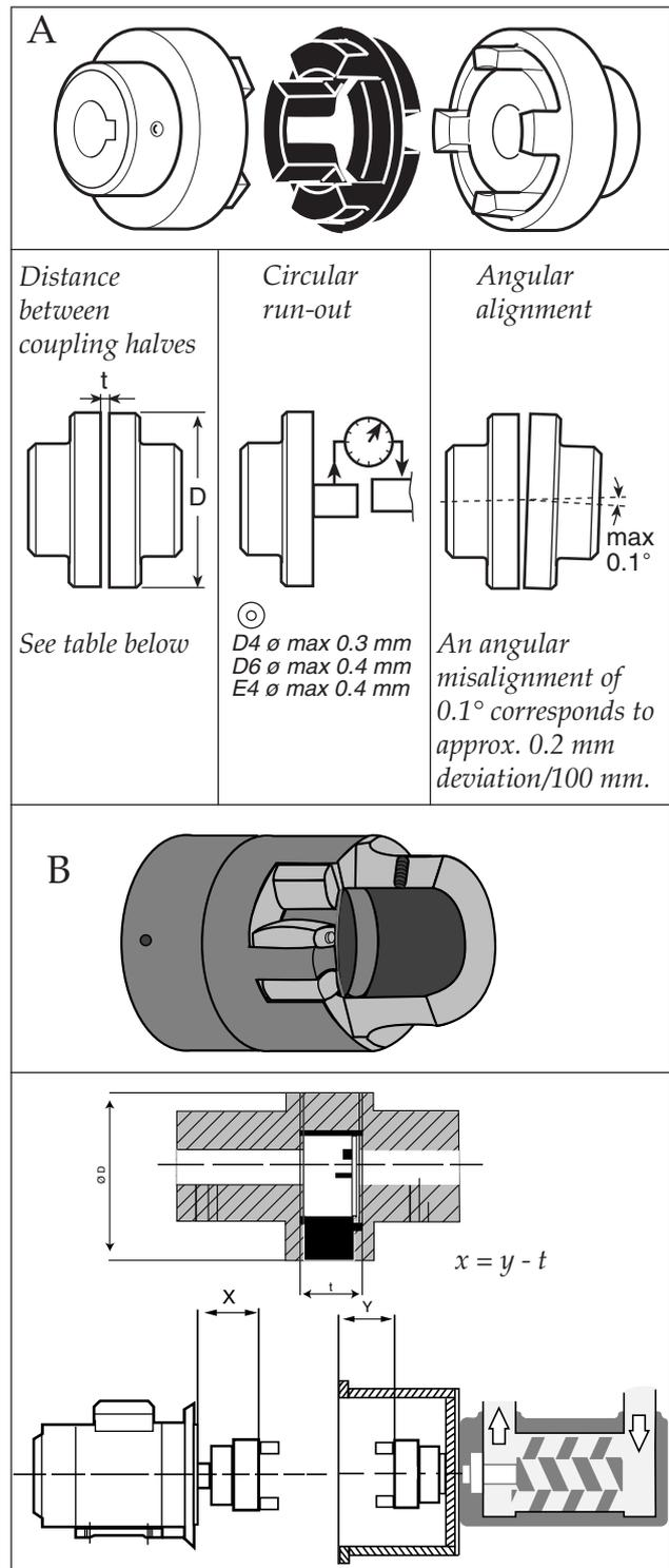
Fig. 3 Alignment of the IMO AB standard coupling
