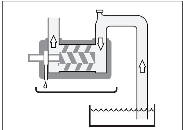
Fig. 10 Shaft seal drain
