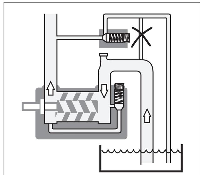
Fig. 14 External control with pressure relief valve
