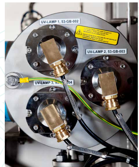
Lamp connection in Ex-safe and service-friendly construction
