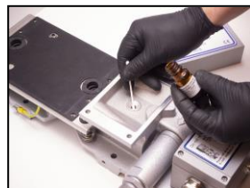
6. clean the large hole in the base plate with cleaning fluid and cotton pins...
