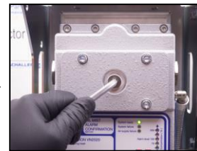
28. remove the quick connection, and the oil mist detector are ready for operation! End of procedure
