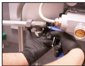
3. blow compressed air into the main pipe for few seconds-so collected oil will drain back to the engine!
