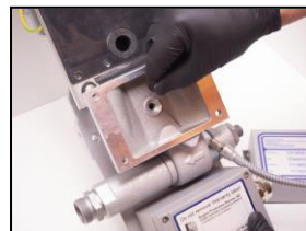
7. use the cleaning needle to open the small hole for dirt and oil...
