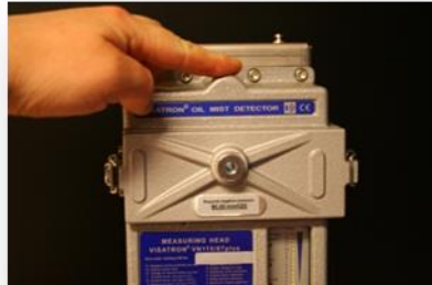
check the heating element if it is hot- if cold device- replace!...
