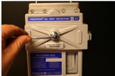
change the screw plug seal 1/4" for inspection cover... (P/n.: 10082)
