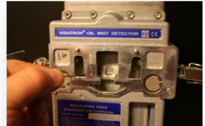
clean the bores with cleaning needle (P/n.: 10135)...
