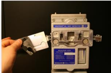
change the seal for inspection cover... (P/n.: 10010/ 10166)
