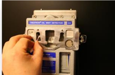
clean the infra- red sensor glasses with cotton sticks and alcohol... (P.n.:10036 & 10035)
