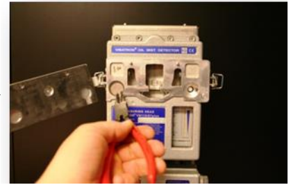
change the scavenging air filter (P/n.: 10042)...
