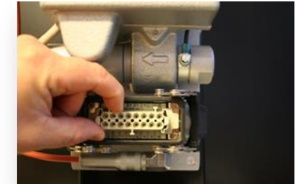
check all leaders in the main socket... If bad condition- replace (P/n.: 10033)
