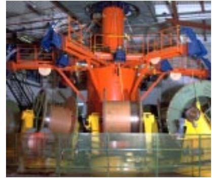
Curing and cooling was changed to take place in a dry atmosphere of pressurized nitrogen. Today Nexans Norway operates a vertical line where the insulation system is extruded on to the conductor by four extruders feeding the material into one extruder head.
