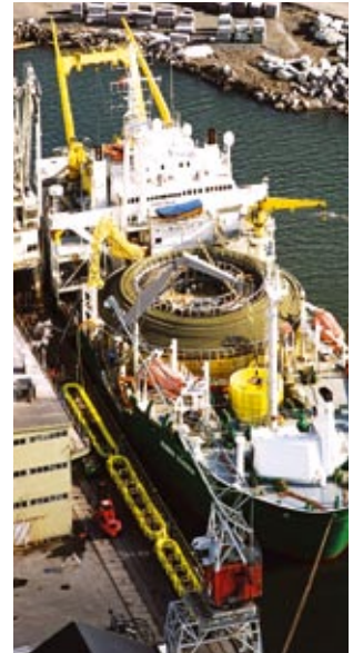
c/s Bourbon Skagerrak loading a fibre optic submarine cable to be installed together with a high voltage cable
