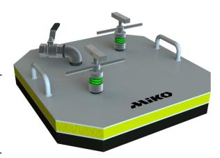
ket will be compressed further. The springs under the wing nuts maintain a constant tension in the rods as this happens, by compensating for the movement of the cover. This means that the divers do not need to go back and re-tighten the wing nuts after emptying the sea chest. Miko's Sea Chest Covers will keep the sea chest dry throughout the entire operation.
