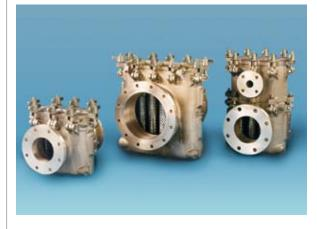
Normally supplied in Gunmetal or Aluminium Bronze with a Cupro-Nickel screen, it is suitable for low or medium pressure applications such as sea water cooling, fire fighting applications, hydraulic and fuel oils and product transfer. The Plenty Seaguard is ideally suited for shock and non magnetic service.
