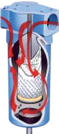
This filter housing cutaway depicts the coalescing process. Air enters the housing and flows through the filter media passing from the inside element surface to the outside. Coalesced liquid, water and oil, collects in the bowl where it is drained and clean air exits the housing through the outlet port. Particulate contaminants are captured and held in the media.
