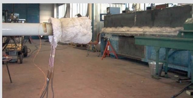
"Heat treatment" of Standpipe Manifold manufactured by Mento Service.
