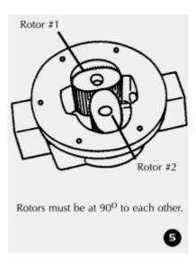
7) Test the meter by turning the rotors with a finger or by applying very low air pressure (no more than a good breath) to one end of the meter, before returning the meter to the line.
