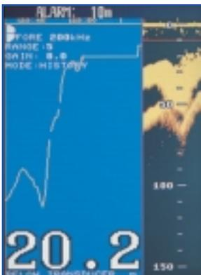
This mode provides a mix of Contour and Strata displays. The Contour display can be shifted back to the past over 24 h while the right side Strata display (layers of different colors according to reverberation strengths) shows the latest five minutes of sounding data.
