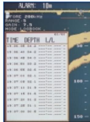
This position of Mode Selector displays the logging on depths and own ship positions with associated time. You can select the time intervals among 5 s, 1 and 2 min options on the Menu. The log book contains 60 pages that can be scrolled up or down with [+] or [-] key. Entry to the logbook is every 5 s over 24 h.
