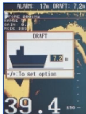
Depth Below Surface mode provides a draft-adjusted depth reading and is useful in referencing to the nautical chart. The draft is adjustable with the [DRAFT] key at the DBS position of the Mode Selector. If you find any difficulty to check for the draft value, use the NAV mode, where you can find the bottom clearance under the keel.
