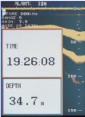
This display mode indicates own ship position, GPS derived course and speed, time and depth in digital form. The user may select the data of particular interest to display in large characters. The screen continues to display the sounding data in the background. Part of graphical indication is visible to the right of data window.
