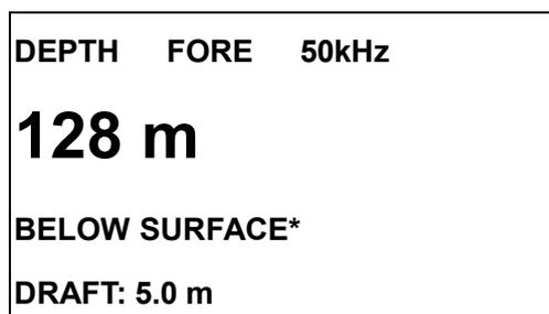
Depth below surface. Draft is determined on the main Display Unit FE-701.
