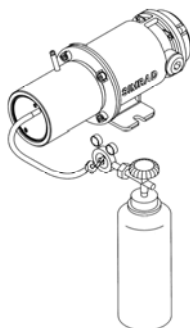
Figure 4.2 Set-up of calibration test
