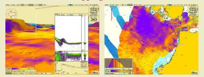
Olex connects to Simrad ES60 and EQ60 echosounders for seabed hardness mapping. The system analyzes the bottom echo, taking into account parameters such as pulse length, beam width and transducer type. A naturalized bottom backscatter is calculated and added to the internal chart. The hardness is shown as adjustable colors from deep pink for soft bottom to bright yellow for hard. The actual echosounder data can also be shown, with present and historic data.
