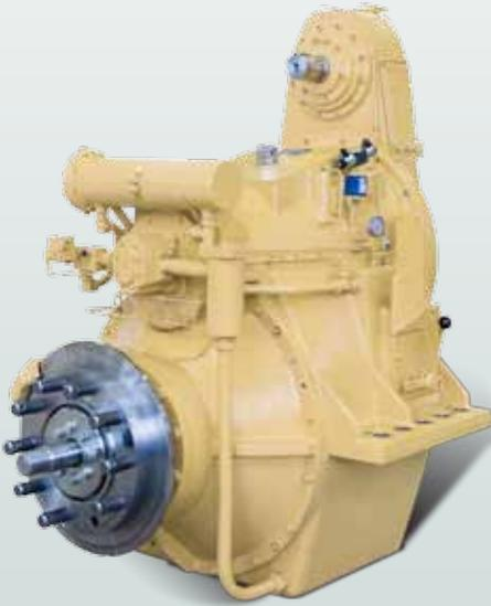
Heimdal reduction gears are produced in seven sizes. Each size may be equipped with various ratios adapted to the engine and propeller speed. All sizes have a built-in servo system for connection to a controllable pitch propeller by means of a pull rod. The gears may be delivered with up to three PTO and/or PTI, and are suitable for both diesel-mechanic or diesel-electric drive.
