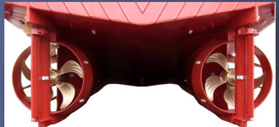
5 blade CP propellers P52, Ø2000mm
