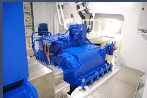
Horizontal gearbox G70HF - Powered by a E motor
