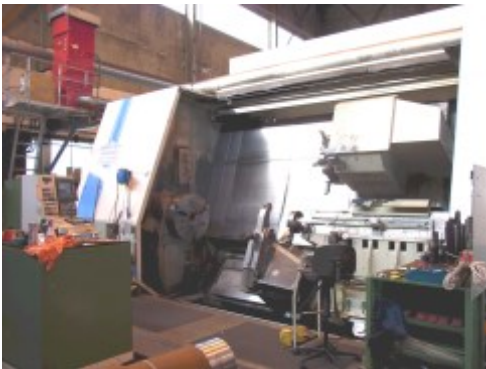
Milling machine : Colgar, x = 22m, y = 5m , z = 2m Table 1 x 120 t + 1 x 30 t Largest in Norway .
