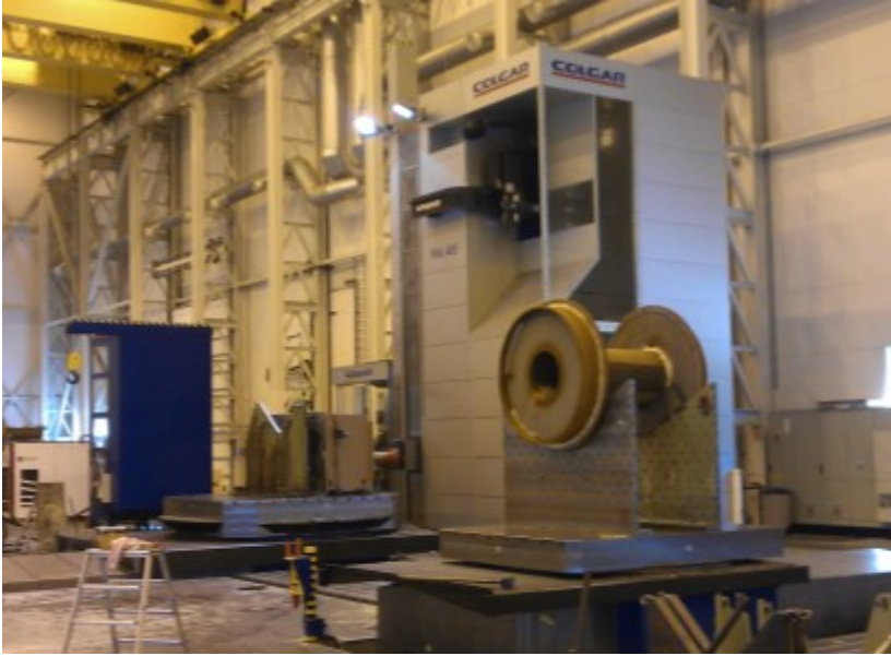
Milling machine : Colgar, x = 22m, y = 5m , z = 2m Table 1 x 120 t + 1 x 30 t Largest in Norway .
