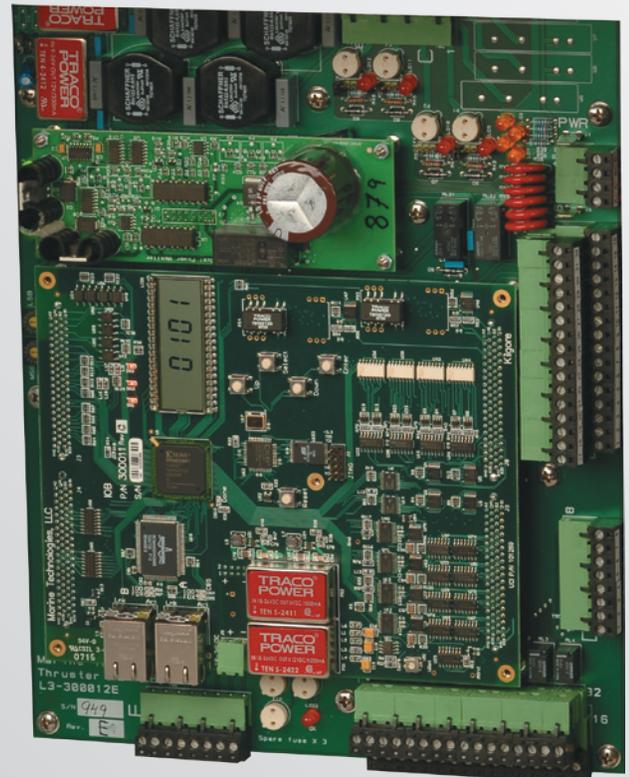
**FIGURE 16 – IO CARD MOUNTED ON A SINGLE THRUSTER INTERFACE MOTHERBOARD**
