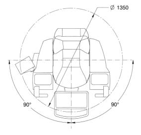
Max. Total rotation 180° with El. Swing/Rotation Art. No. 6555 Max. Total rotation 180° with Standard option of Manual Swing/Rotation
